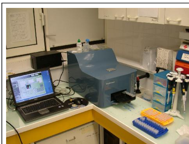
Figure 1: Bench-top, portable GUAVA EasyCyte Plus flow cytometer transported from LEMAR and temporarily operated in IRIS facilities in April 2008.
