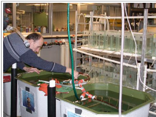
Figure 2: Mussels were exposed in tanks dosed with selected contaminants in IRIS facilities
